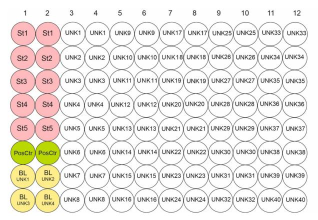
**Plate layout for NAD+ assay:** St – standard, BL – blanks with indicated samples used for the blank reading, UNK – unknown samples, stabilized extracts from the samples with unknown metabolite concentration, PosCtr – stabilized Positive control. Use 20  $\mu$ L of standards, Positive control, and stabilized sample extracts per well. Sample blanks of the first four samples are analyzed in the master mix without added enzyme.
